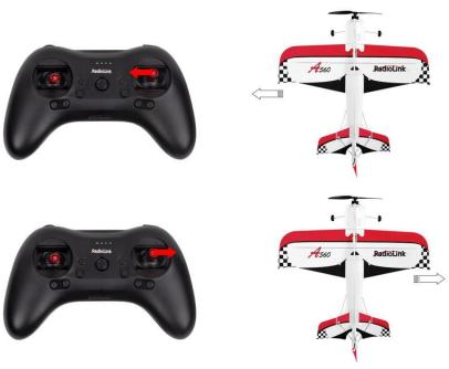
When the A560 is vertical, toggle the elevator joystick(CH2) to control the A560 moving forward or backward.
