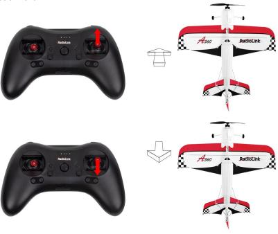
When the A560 is vertical, toggle the rudder joystick(CH4) to control the aircraft moving left or right.
