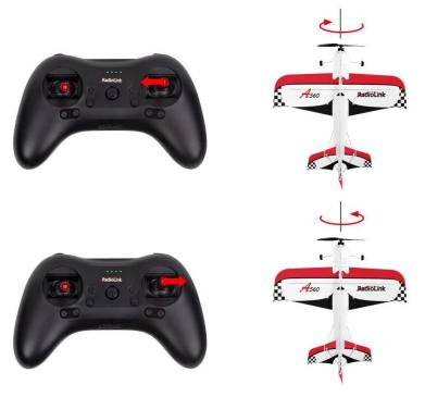
When the A560 is vertical, toggle the elevator joystick(CH2) to control the A560 moving forward or backward.
