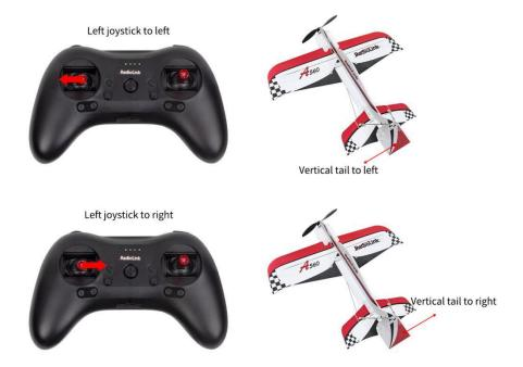
In manual mode, operate the joystick of the transmitter. If the movement of the control surface of the corresponding channel is reversed, enter the setting page of the transmitter to adjust the transmitter phase of the corresponding channel.
