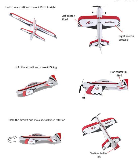
In Stabilize Mode, if the gyro phase is reversed, please adjust the gyro phase by the flight controller Byme-A V2.0. See the below chapter for the adjustment method.
