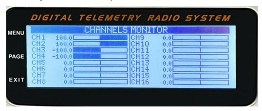
CH1 2000 µs (opentx +100), CH2 2000 µs (opentx +100) CH3 1000 µs (opentx -100), CH4 1000 µs (opentx -100)
