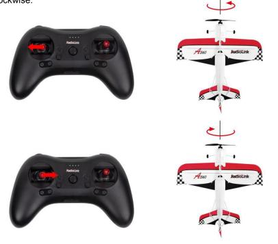
If the throttle joystick is toggled upward, the A560 climbs upwards at a vertical attitude. If toggled downward, the A560 descends at a vertical attitude.
