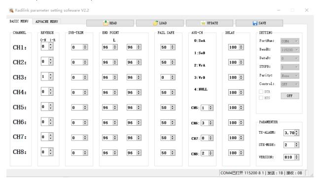
**REVERSE**: Defines the relationship between the transmitter controls and the receiver output for channels with option of NORM and REV. Refer to 3.3.2-**REV** (P7) for more details.
