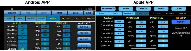
Different from the current Apple App, the current **Android APP** has two more programmable mixing controls, Throttle Curve and DR Curve parameter setup menus and customizable RSSI/Model Voltage Alarm.
