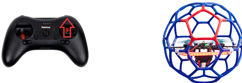
Pitch stick upward, LD-B20C moves forward
