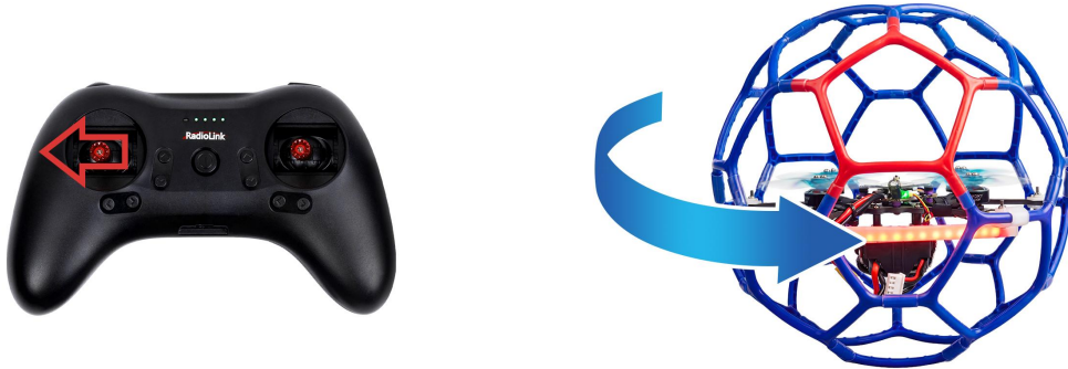
Yaw stick to the left, LD-B20C turns anticlockwise
